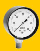
Trerice Low Pressure Gauges are essential for accurately measuring low pressures such as natural gas. This gauge employs a diaphragm capsule element to accurately measure pressures of 10 psi or below. The case is drawn steel with brass wetted parts.
