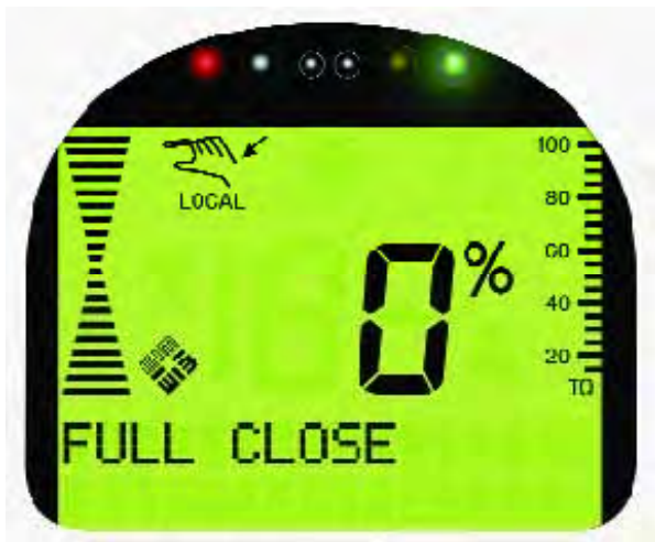
TEC2000 ICONOTEXT DISPLAY showing actuator in LOCAL mode and valve in full close position.
