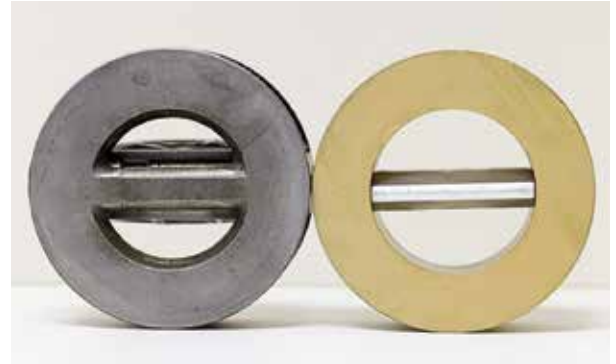
Our elastomer hinge design (on right) eliminates the check valve seat, provides greater open area and lower pressure drop compared to traditional metal hinge dual plate wafer check valves.
