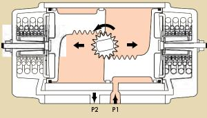
For counterclockwise output, apply pressure to P1, which forces the pistons apart and compresses the springs. The linear travel of the pistons is converted to a rotation of the drive shaft by rack to pinion connection. The volume outside each piston is exhausted at P2
