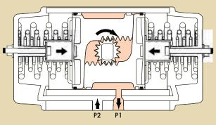
For clockwise output, the volume between the pistons is exhausted to P1, causing the springs to force the pistons together. Air is admitted through P2 as pistons move together.
