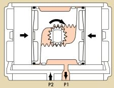
For clockwise output, apply pressure to P2, which forces the pistons to move together. The volume between the pistons is exhausted at P1. The linear travel of pistons is converted to rotation of output shaft by rack to pinion connection.
