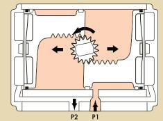
For counterclockwise output, apply pressure to P1, which forces the pistons apart. The linear travel of the pistons is converted to a rotation of the output shaft by rack to pinion connection. The volume outside each piston is exhausted at P2.
