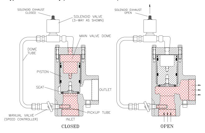
The FLOW SAFE F70U Series unloader valve provides a means to control flow for a variety of process flow applications, such as compressor and blower unloading. It is designed to be repeatedly cycled at full pressure throughout its range of rated temperatures.
