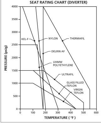
Extended pressures and temperatures may be achieved by alterting design for specific applications. Consult factory with service conditions. **The valve rating is the lesser of the body rating and the seat rating.** TBV manufactures an extensive line of high pressure valves capable of the full seat ratings shown. Consult factory for details.
