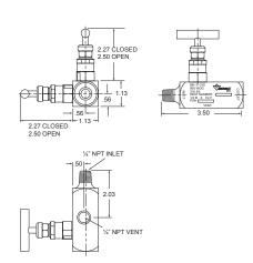
The Versa Block and Bleed valve is a traditional isolation valve. It consists of "block" and "vent" needle valves to isolate and vent downstream pressure during gauge changes.
