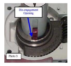
Step 4. Rotate the SRD input shaft CCW until the key in the drive coupling comes into contact with the end of the key slot and the coupling just begins to turn. (Ref Photo 2). Upon contact, reverse the SRD input shaft ½ to ¾ of a turn to disengage the drive coupling key from the worm wheel. This will put a very small opening between the key slot and the drive coupling key. This is the SRD unit's **Home Position**. (Ref Photo 3)
